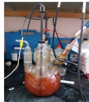
**Figure 3.** Corrosion cell
