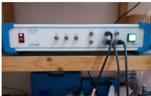
**Figure 2.** Potentiostat Voltalab 10
