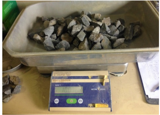
Figure 5. Initial weighting of the test sample
