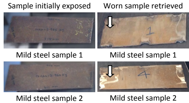
Figure 9. Mild steel samples visual comparison (arrow indicates the direction of the bulk material flow on the sample)
