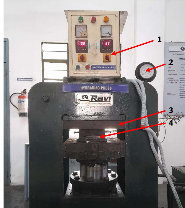
Figure 2. Hydraulic press with brake pad die: 1 – temperature control knob and display; 2 – hydraulic pressure gauge; 3 – heating coil; 4 – brake pad die
