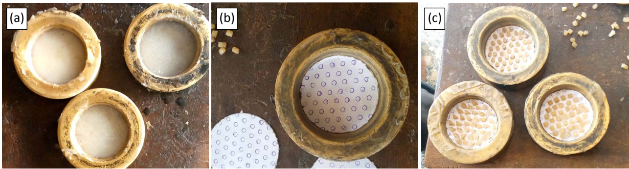
Figure 2. Moulds preparation: (a) moulds with thick slurry applied, (b) texture pattern positioned in mould and (c) beeswax dimples positioned in moulds
