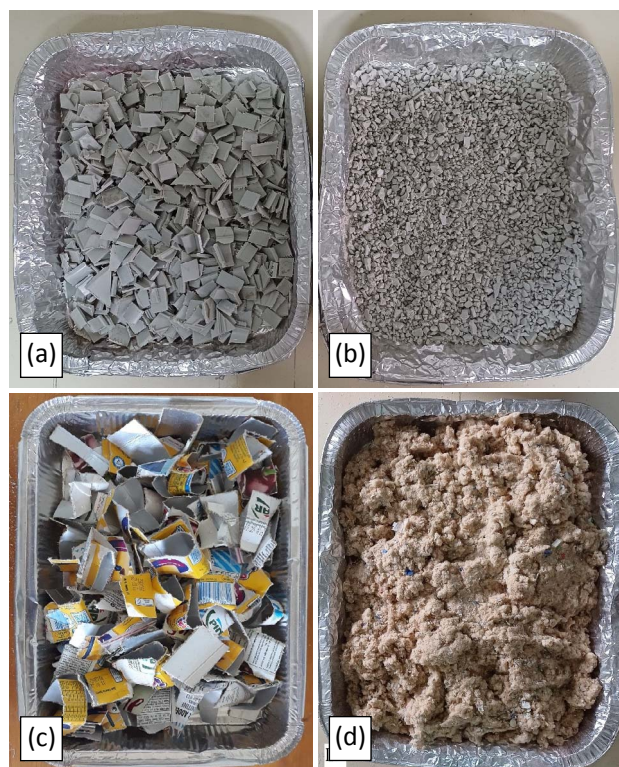
Figure 1. Materials: (a) waste plastic chairs pieces, (b) ground waste plastic chairs pieces, (c) shredded TPBs and (d) ground TPBs
