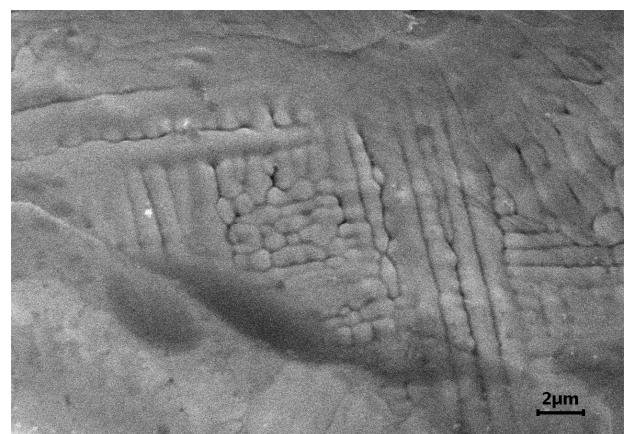
Figure 8. SEM image of dendritic structures seen on the surface of the 3D printed sample at 6000×, BSED
