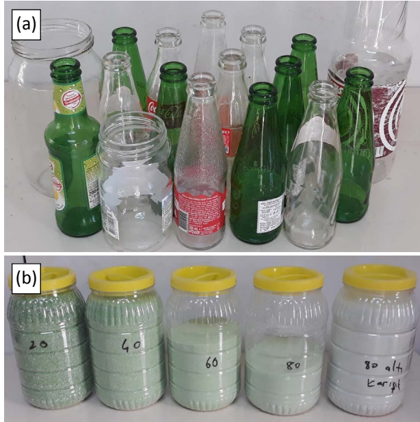
Figure 1. Materials: (a) waste glass bottles and (b) sieved waste glass powders
