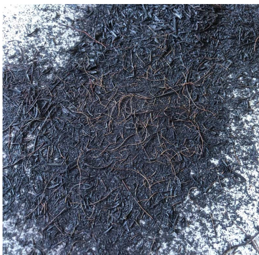
Figure 9. Residual coil wires noticed in the slag after 15-minute test thermal pretreatment
