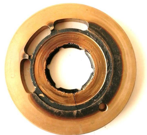
Figure 1. Worn thrust bearing
