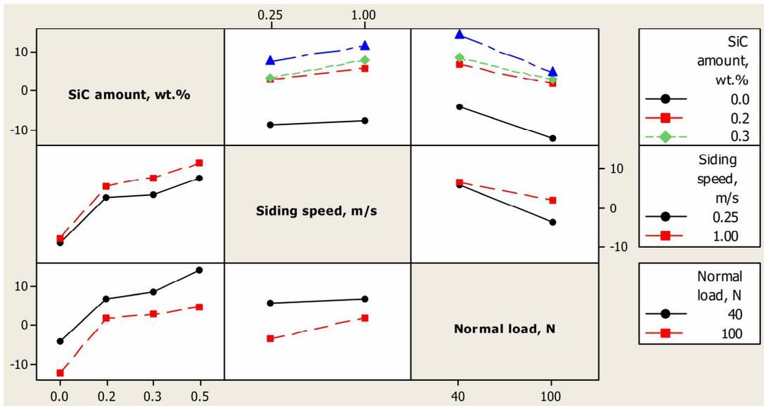
**Figure 4.** Interaction plot for S/N ratios (smaller-is-better characteristic)
