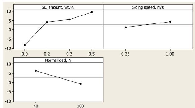
**Figure 3.** Main effects plot for S/N ratios (smaller-is-better characteristic)
