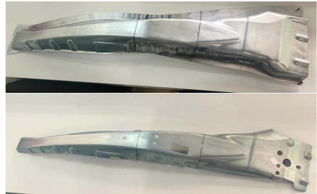
**Figure 2.** Formed welded sheet metal
