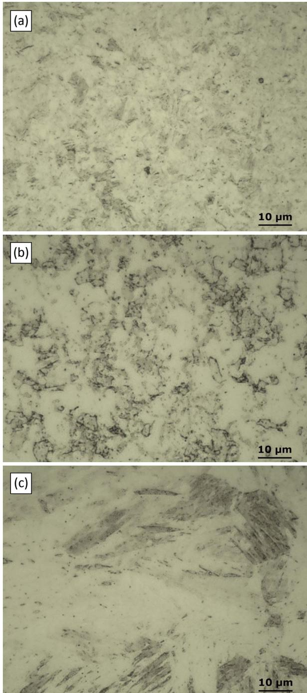
**Figure 6.** Microstructure visuals of different areas: (a) HAZ, (b) formed part and (c) HAZ of the formed part; optical microscope images at 1000 × magnification
