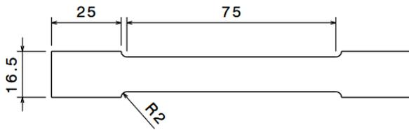
**Figure 3.** Sizes of the tensile testing samples
