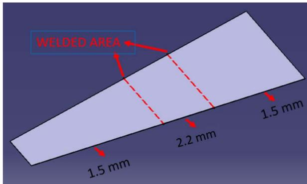
**Figure 1.** Welded sheet metal physical model
