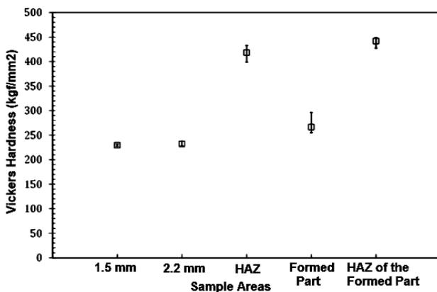
**Figure 11.** Vickers hardness values of samples taken from different areas
