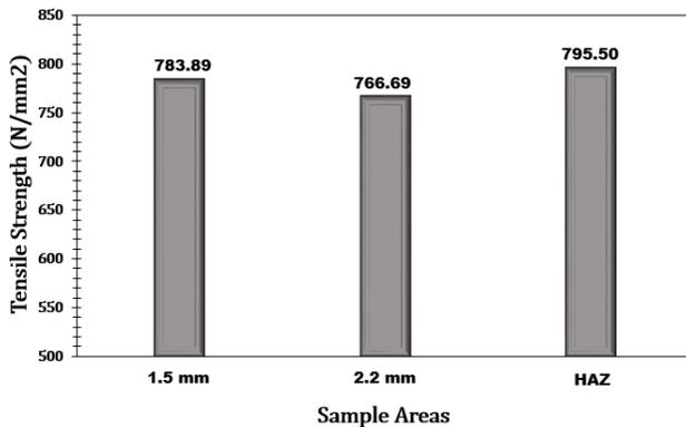
**Figure 7.** Tensile strength values of samples taken from different areas
