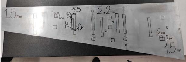
**Figure 4.** Study of obtaining the tensile testing samples
