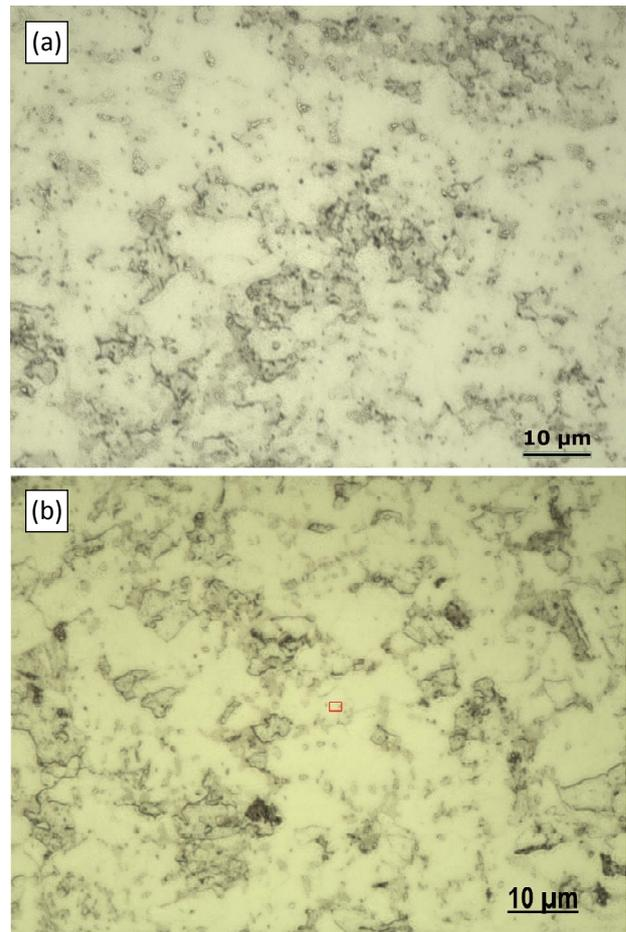
**Figure 5.** Microstructure of samples with different thicknesses: (a) 1.5 mm and (b) 2.2 mm; optical microscope images at 1000 × magnification
