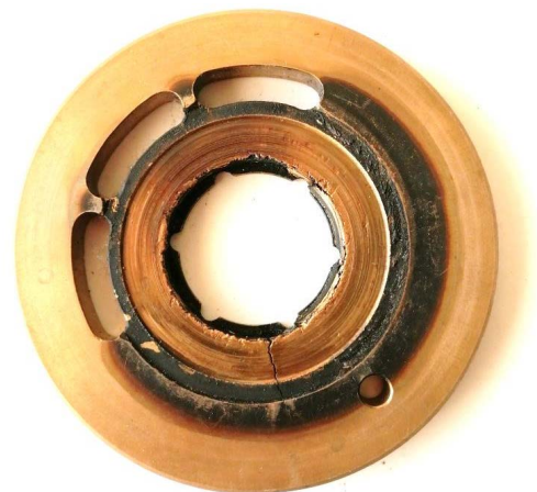
Figure 1. Worn thrust bearing
